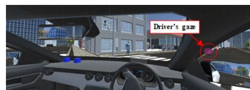
Figure 11. Dangerous situation that occurred without HMI. (The driver kept his eyes on the preceding vehicle and passed through the intersection without noticing the pedestrian who had started walking.)
