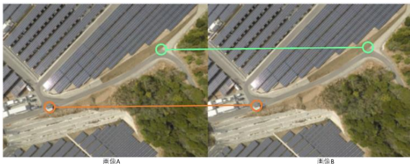
(a) (b) Extract Feature point and matching (This image is simulated.)
